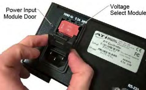
Figure 2.8—Removing Voltage Select Module
